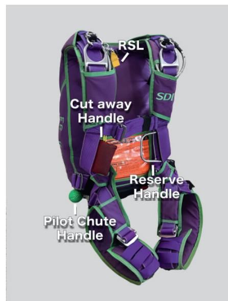
**Handles must be activated in the correct order in the event of a malfunction.**
