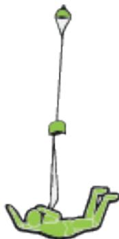
once all the lines are unstowed the deployment bag opens and the canopy is extracted.
