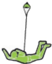
pilot chute and bridle extract the deployment bag and the lines unstow from rubber bands on the deployment bag
